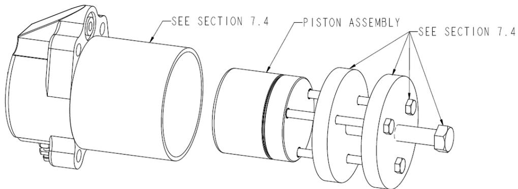
8.3.7 Use snap ring pliers to remove snap ring (15) from piston assembly.
