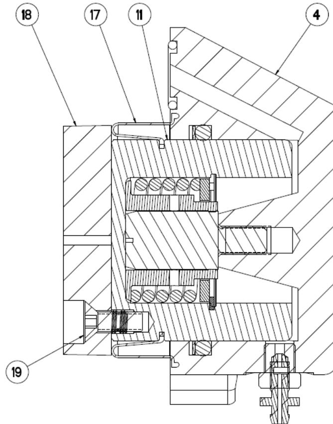
8.3.28 Install the piston housing assembly with four screw (5) and washers (6). Apply Loctite NO.242 sealant to threads and torque to 43-45 LB-FT.
