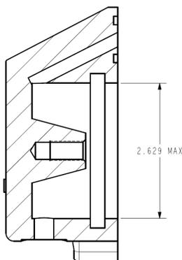
8.3.13 Inspect guide (8) in the piston housing (4) for excessive wear. Use crocus cloth to remove light scratches and corrosion from outer diameter of the guide (8). Use a flat blade screw driver or 6mm hex key or socket to remove and replace guides that measure less than .7515 INCH in diameter. Apply Scotch-Weld No. 2158 B/A adhesive to the threads and torque to 130-145 LB-IN. allow 12-24 hours for adhesive to set.
