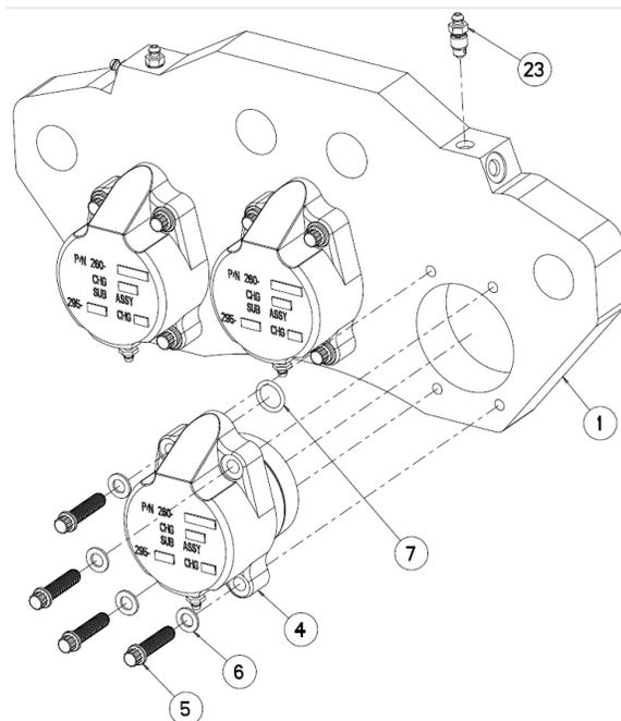
8.3.3 Remove and replace any damaged or corroded bleeder valves (23) in the torque plate(1).
