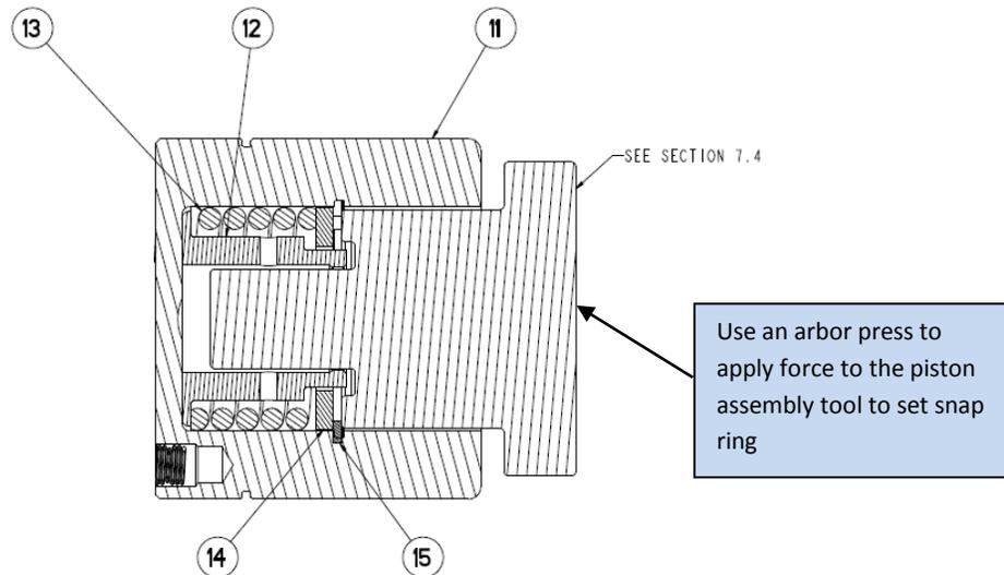
**Note:** A suitable tool of the customer's choice can replace the piston assembly tool.
