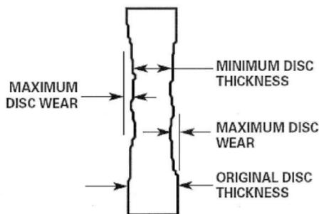
TYPICAL SECTION THROUGH DISC SHOWING
