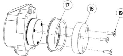
8.3.6 Remove the piston assembly from the piston housing (4) using a suitable puller. See Section 7.4 for an example.
