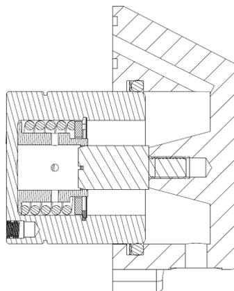
8.3.22 Use an arbor press or a suitable C-Clamp to bottom the piston in the piston housing bore.
