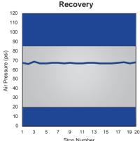
Testing conducted in accordance with F.M.V.S.S. #121 criteria @ 23,000# axle load: 16 1/2 x 7" S-cam air brake; 30 x 5.5" input power and a 20.8" tire rolling radius. Shaded area indicates non-compliance.
