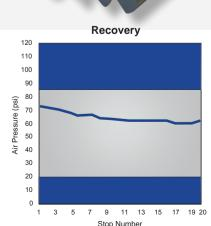
Testing conducted in accordance with F.M.V.S.S. #121 criteria @ 20,000# axle load: 16 1/2 x 7" S-cam air brake; 30 x 5.5" input power and a 20.8" tire rolling radius. Shaded area indicates non-compliance.
